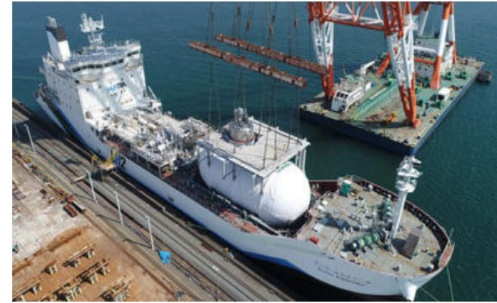
LH2 storage tank for marine transportation
